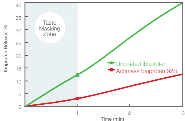
Figure 1. At oral pH, very low active release of Ibuprofen in the first minute demonstrates good taste-masking.
